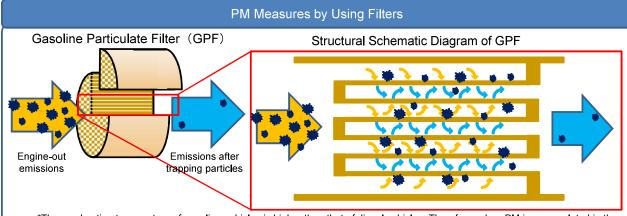
\*The combustion temperature of gasoline vehicles is higher than that of diesel vehicles. Therefore, when PM is accumulated in the filter, natural regeneration occurs by burning PM during fuel cut due to deceleration. However, additional measures are necessary when the temperature required for PM combustion is not achieved or when sufficient amount of oxygen is not secured for combustion, such as during continuous low-speed driving.
